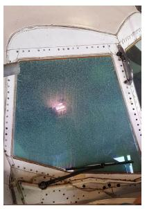
The new windscreen was originally supplied by Brooklands Museum in 2011; the windscreen was cracked when supplied, but GKN, who manufactured the glass panels, repaired it in 2011, and since then it has been in safe storage at Manchester. This windscreen was lifted up to the working platform height. It was fitted to the aircraft, cleaned, and set correctly so the frame fitted. It was then a simple task of replacing all parts; frame screws were not
